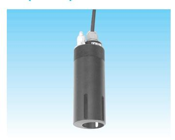
The Turbidity probe TU 8182 has been designed for submersible applications. It is provided with a built-in device for cleaning the optical lens by means of pressure air blasts.
