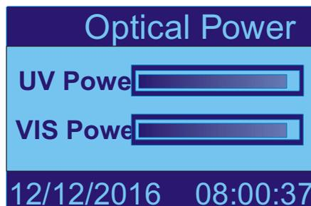
The "UV Power" level bar indicates the power of the UV LED.
