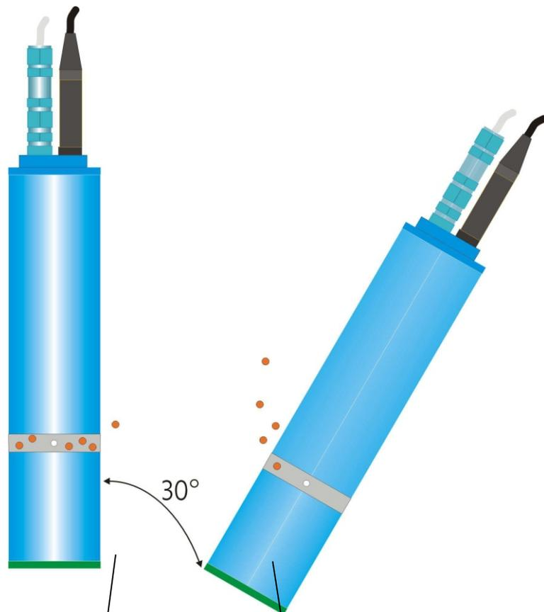
**When vertical,** air bubbles can remain lodged and throw off the measurements
